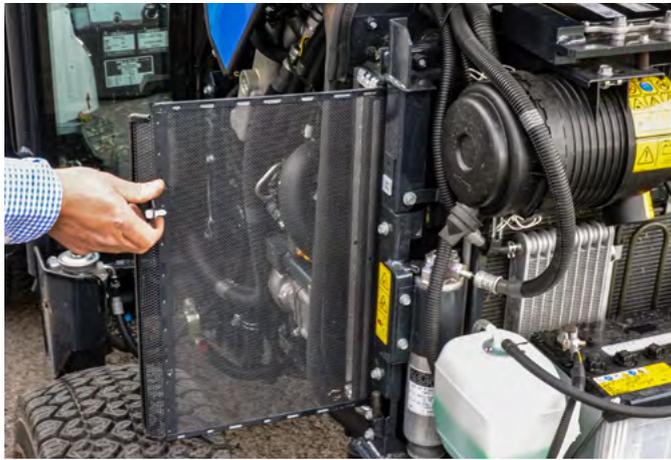
The TH5 range has ISEKI's newly developed Stage V compliant engine, fitted with common-rail injection and exhaust after treatment.
